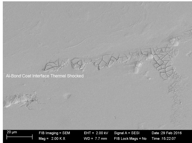
Figure 7. SEM cross section micrograph of TBC on thermally stressed surface revealing cracks the aluminium-bond coat interface.
