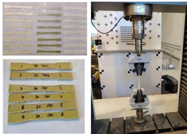
Figure 4. Tensile specimens of fiber glass and Kevlar, Tensile test
