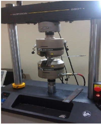
Figure 14: INSTRON Machine setup manufactured specimens.
