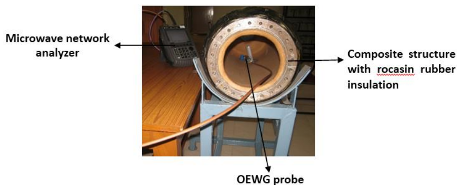
Figure 9. Experimental setup for inspecting composite pressure vessel with rocasin rubber insulation by contact method at Ku-band
