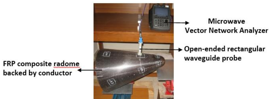
Figure 13. Experimental setup for inspecting composite radome by non-contact method at Ku-band
