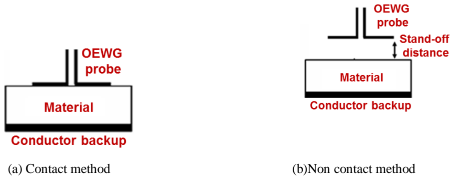
Figure 1. Near-field reflection microwave NDE test configuration
