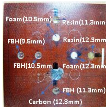
Figure 17. Configuration of E-glass epoxy composite with multiple defects (flat bottom holes: empty, carbon fabric, foam and resin)
