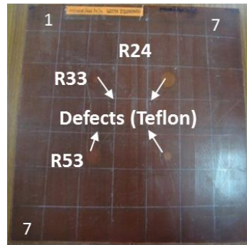
Figure 5. Configuration of E-glass epoxy composite with Teflon inserts
