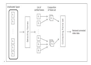
Fig. 3.1. Processing steps of the proposed frame-based video file restoration technique.
