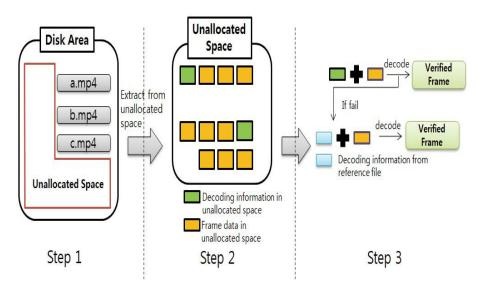
Fig. 3.2. The procedure of video file restoration using video file format specifications.
