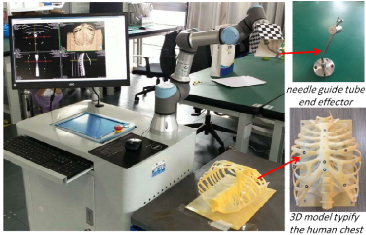
Figure2. Experimental setup, showing the GUI, 3D chest model and needle guide tube end-effector
