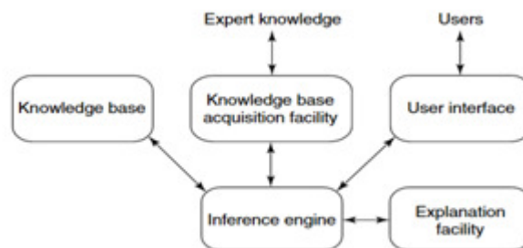
FIGURE 2:Architecture of a simple expert system. [6]
