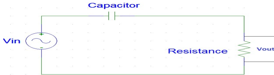
Fig:6 Capacitive high pass filter circuit
