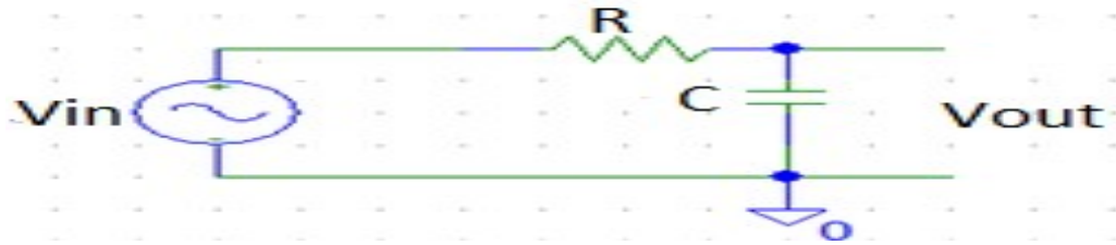
Fig.4: Circuit diagram of low pass filter
