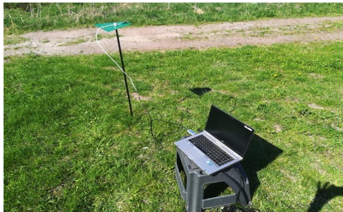
Figure. 2. An overview of the portable RFI measurement system. The system is consisting of log periodic circuit board antenna, SDR-RTL dongle and control computer.
