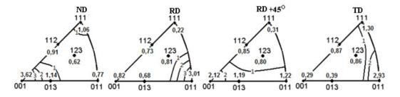
Figure 2. IPF of sheet of alloy Fe - 3% Si after direct rolling to a thickness of 1.5 mm
