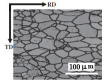
Figure 6. The microstructure of sample of alloy Fe -3 % Si after transverse rolling and subsequent annealing
