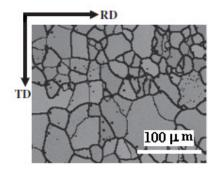
Figure 4. The microstructure of initial sample of alloy Fe – 3 % Si
