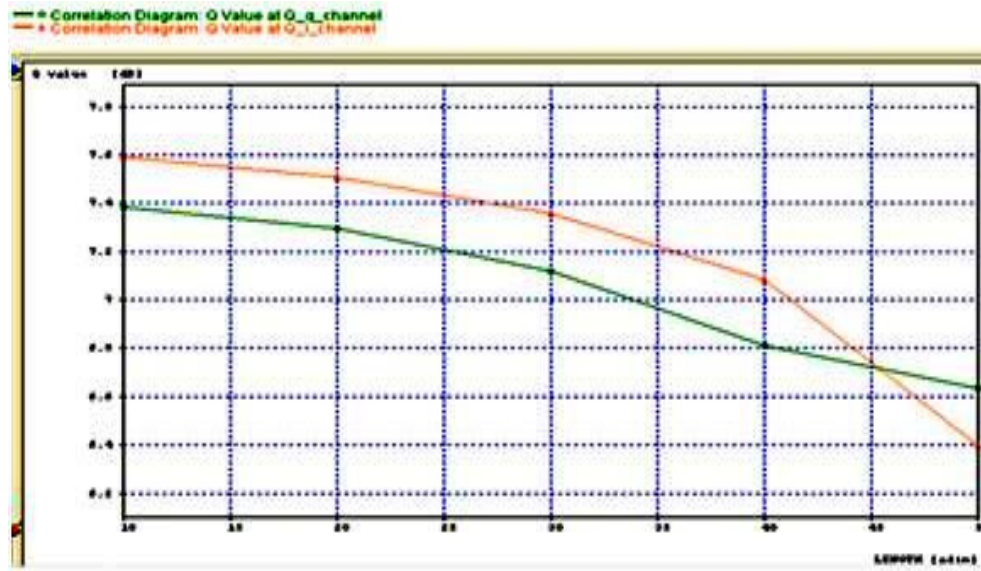
Figure8: Q vs. Length OOFDM (bit rate 10Gbps, baud rate2.5, subcarrier32, CP0.99)
