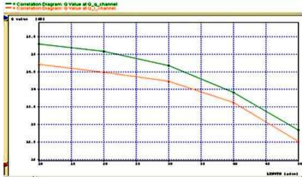
Figure6: Q vs. Length (50km) OOFDM (bit rate 5Gbps, baud rate2.5, subcarrier16, CP0.99)
