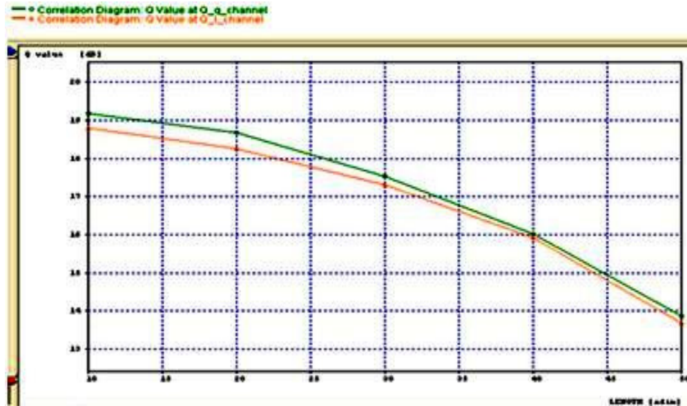
Figure4: Q vs. Length (50KM) simulated OOFDM (bit rate 5Gbps, baud rate2.5, subcarrier8, CP0.99)
