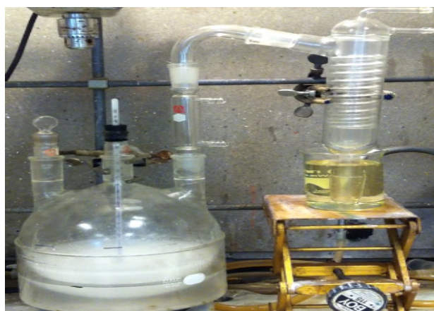
Figure 1. SPDPC synthesis and HCl neutralization setup.
