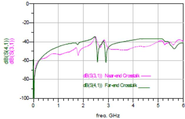
Figure.9. Simulation Results of Near and Far end Coupling for Non-Parallel Microstrip lines with Via fence in Inclination is 300
