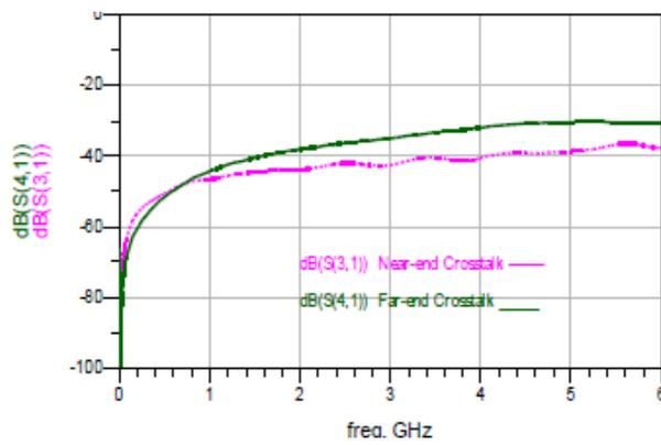
Figure.10. Simulation Results of Near and Far end Coupling for Non Parallel Microstrip lines in Inclination is 450
