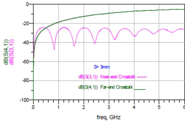
Figure.6. Simulation Results of Near and Far end Coupling for Parallel Microstrip lines in Spacing  $S=3$  mm
