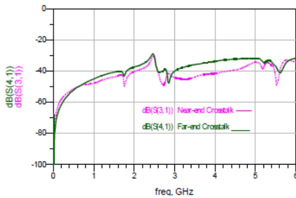
Figure.11. Simulation Results of Near and Far end Coupling for Non Parallel Microstrip lines with Via fence in Inclination is 450
