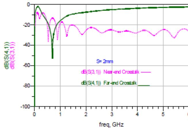
Figure.5. Simulation Results of Near and Far end Coupling for Parallel Microstrip lines in spacing  $S=2$  mm
