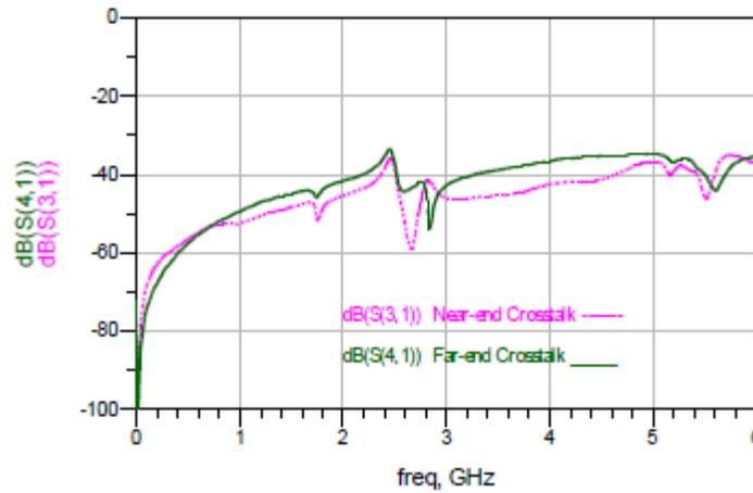
Figure.13. Simulation Results of Near and Far end Coupling for Non Parallel Microstrip lines with Via fence in Inclination is 600
