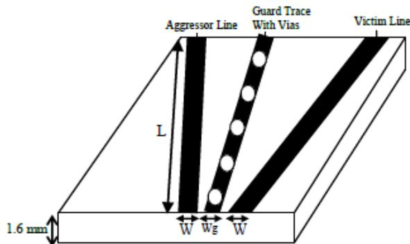
Figure.4. Non-Parallel Microstrip lines with Via Fence
