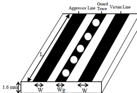
Figure.2. Guard Trace and Grounded Vias
