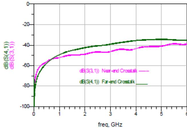
Figure.12. Simulation Results of Near and Far end Coupling for Non Parallel Microstrip lines in Inclination is 600
