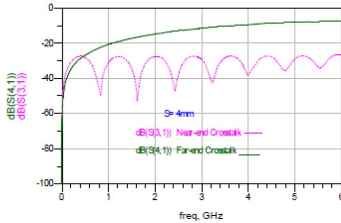
Figure.7. Simulation Results of Near and Far end Coupling for Parallel Microstrip lines in Spacing  $S=4$  mm
