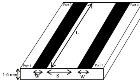
Figure.1. PCB Structure With Two Microstrip lines
