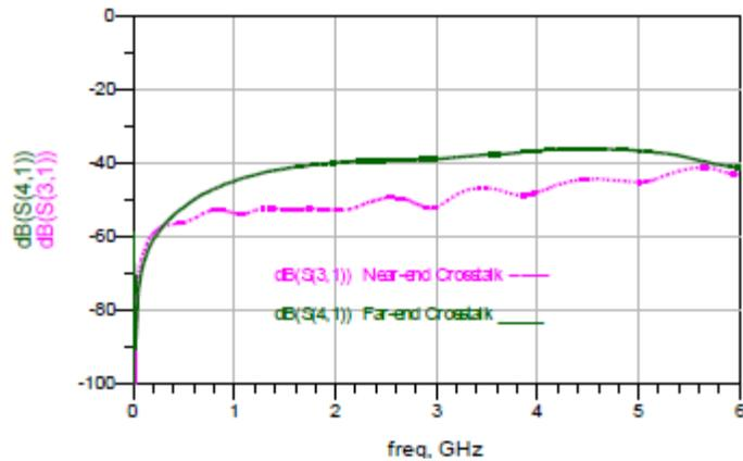
Figure.8. Simulation Results of Near and Far end Coupling for Non Parallel Microstrip lines in Inclination is 300
