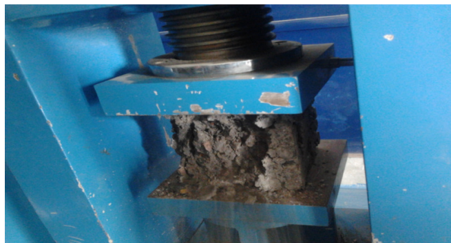
Figure 1: Cube under compression machine
