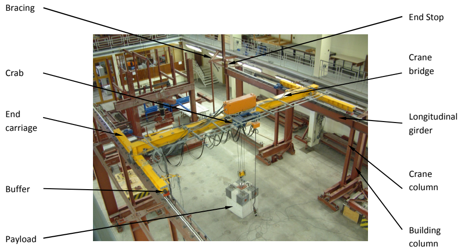
Figure 1: A 5 ton single-top running electrical overhead travelling crane
