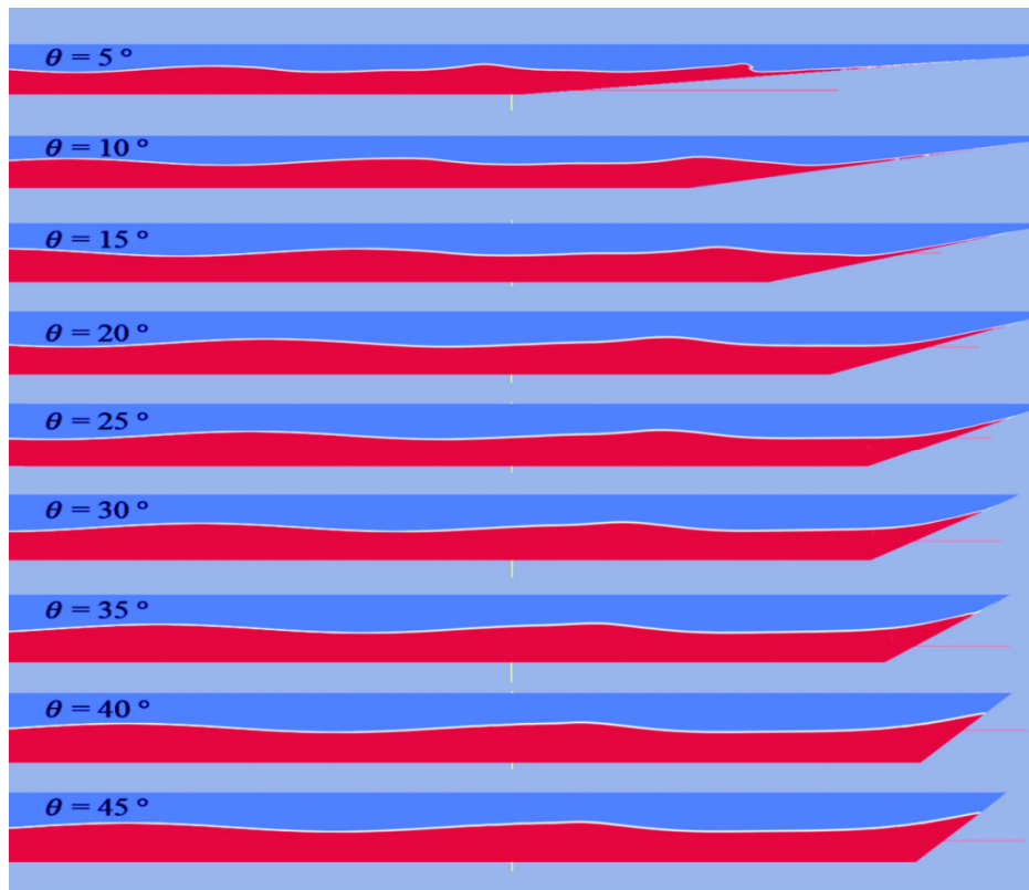
Fig.2. Airy wave run-ups on different slopping beds, ranging from 5 to 45 degrees.
