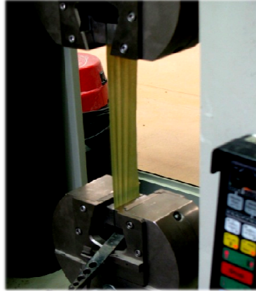
Figure 4: The universal testing machine used for tensile testing of polyethylene
