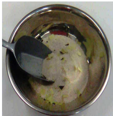
Figure 5: Randomly mixed sand-plastic composite for testing.
