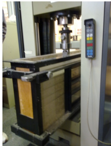
Figure 10: Loading box placed in Zwick Machine
