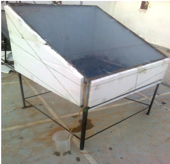
Figure 2: Final stage photograph of solar still
